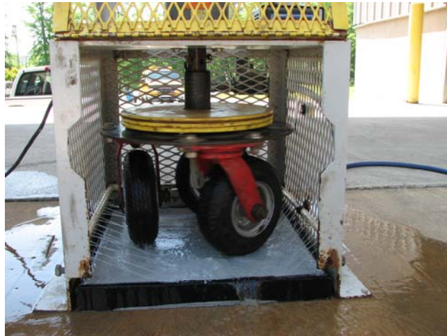
FIGURE 2 Polishing E-Krete® surface using TWPD in laboratory.
