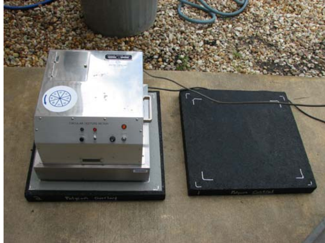
FIGURE 4 Circular Texture Meter on E-Krete ® surface next to HMA.
